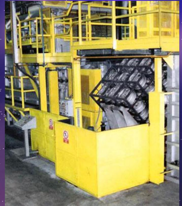
Aluminium Heat Treatment Furnace Type I T6
