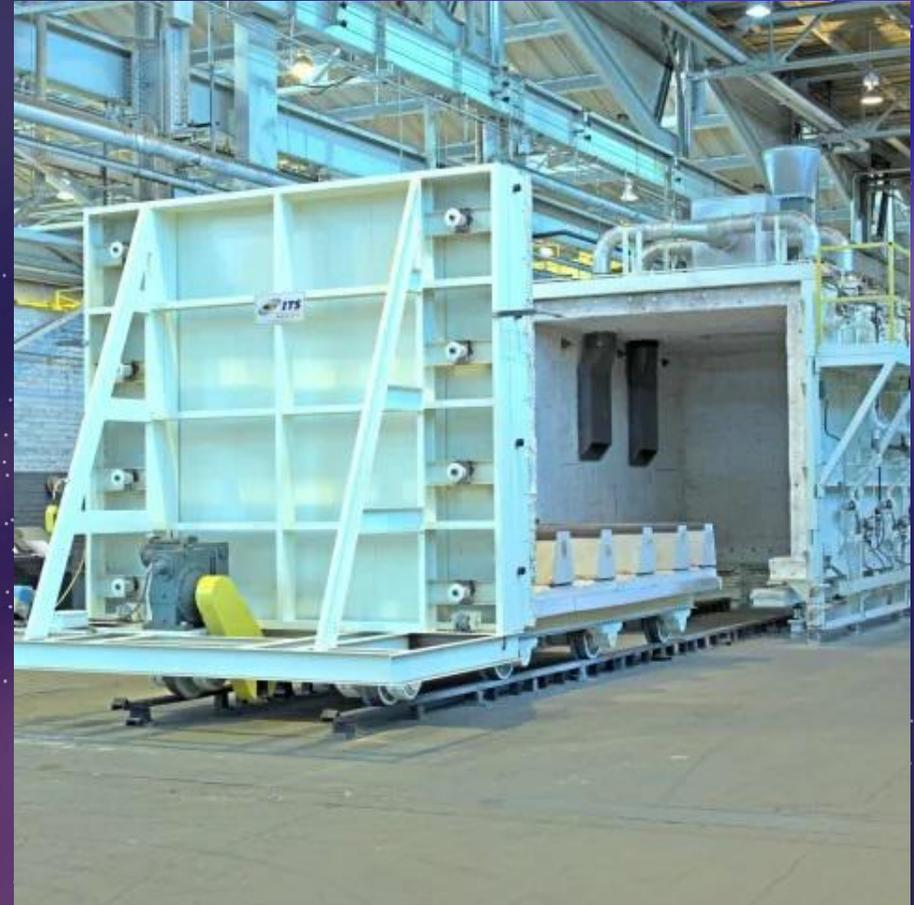
Aluminium Heat Treatment Furnace Type I T6
