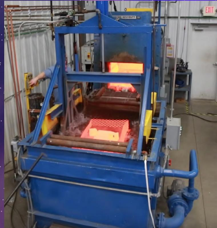
Aluminium Heat Treatment Furnace Type I T6
