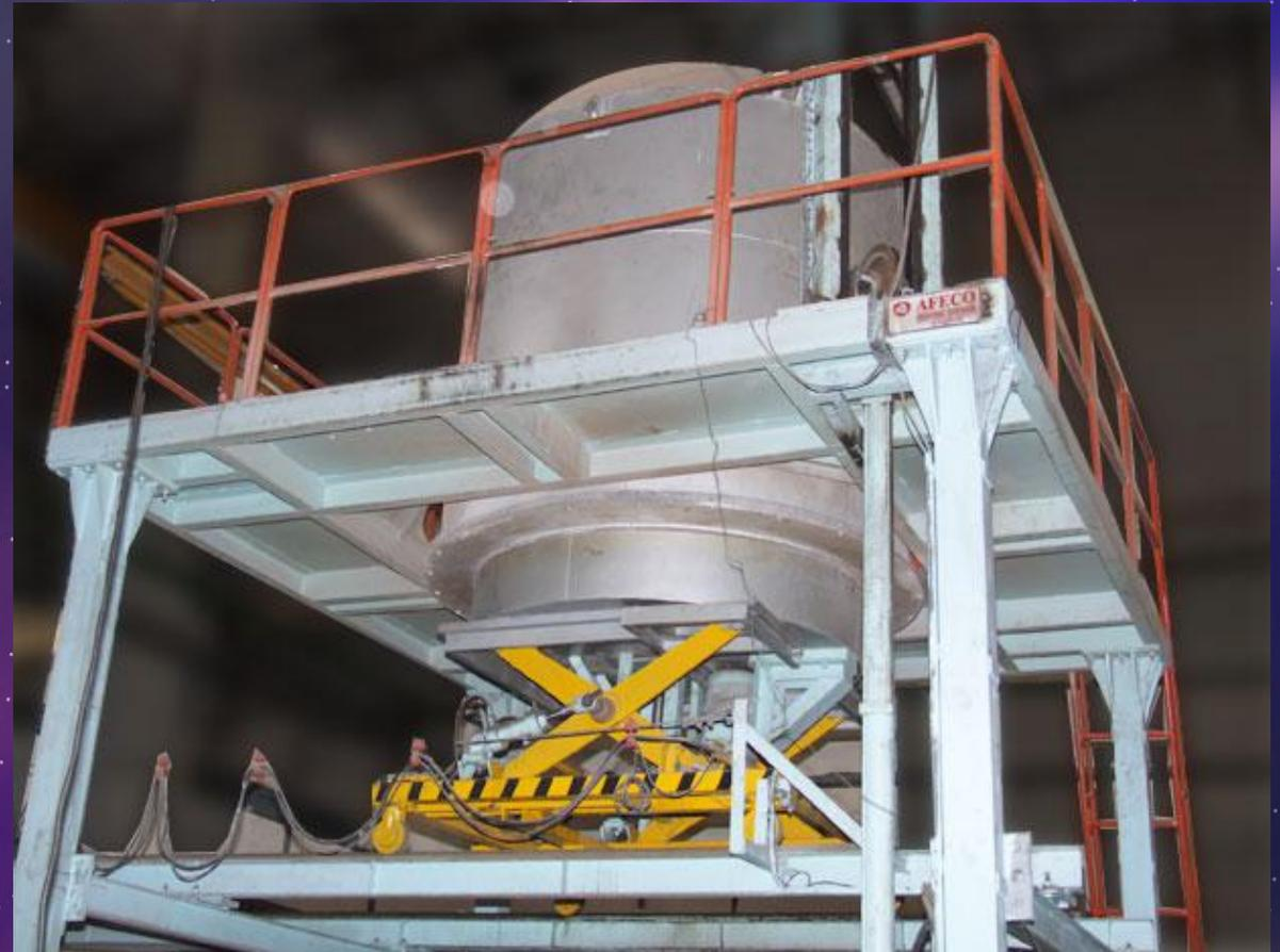
Aluminium Heat Treatment Furnace Type I T6
